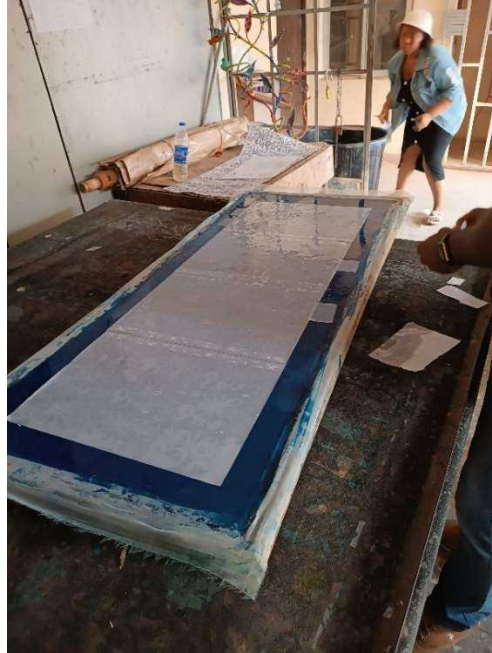
Plate 4: Attaching the paper to the coated screen
