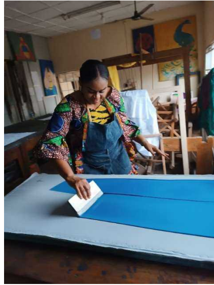
Plate 1d: Coating of the screen
