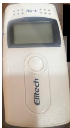
Figure 2a: Elitech RC -4 temperature data logger used for attic and indoor temperature measurements Source: Fieldwork (2025)
